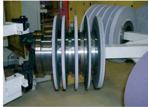
Ill.: Grinding wheel magazine and wheel-changing device
